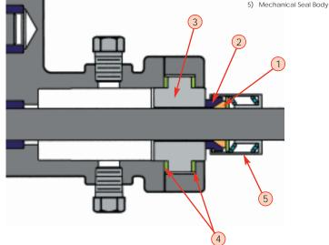
The **External Mechanical Seal** arrangement is used when system pressures are below atmospheric pressure (vacuum). This is because the atmospheric pressure will assist in holding the seal faces together. This seal arrangement isolates the mechanical seal from the fluid being pumped which can be an advantage when pumping chemicals that are not compatible with the seal body. The maximum fluid viscosity recommended is 5000 CPS.
