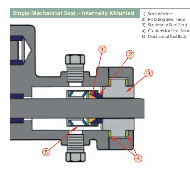
The **Single Mechanical Seal** arrangement is the standard and is by far the most commonly used when pumping any type of chemical where leakage needs to be kept to a minimum. This seal type can tolerate limited amounts of abrasive particles. The maximum fluid viscosity recommended is 5000 CPS.
