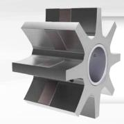
A special ribbed idler gear was developed for massecuite and magma. This idler ensures that 80% of the gear flank does not contact the rotor gear, to ensure that crystals are not damaged by gear contact.
