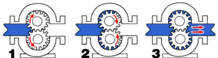
1. As the gears come out of mesh, they create expanding volume on the inlet side of the pump. Liquid flows into the cavity and is trapped by the gear teeth as they rotate.
