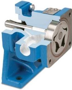
Gerotor pumps are [internal gear pumps](#) without the crescent. The rotor is the internal (drive) gear shown below in gray, and the idler is the external (driven) gear, shown below in orange. They are primarily suitable for clean, low pressure applications such as lubrication systems or hot oil filtration systems, but can also be found in low to moderate pressure hydraulic applications.
