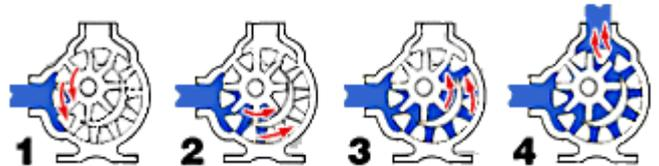
2. Liquid travels through the pump between the teeth of the "gear-within-a-gear" principle. The crescent shape divides the liquid and acts as a seal between the suction and discharge ports.
