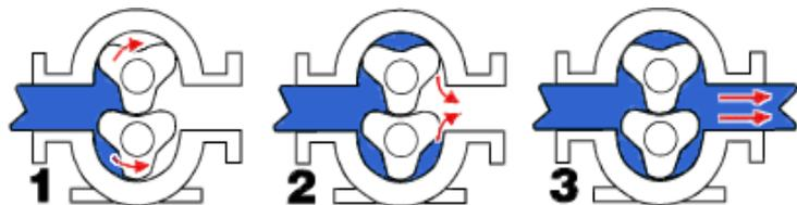
1. As the lobes come out of mesh, they create expanding volume on the inlet side of the pump. Liquid flows into the cavity and is trapped by the lobes as they rotate.
