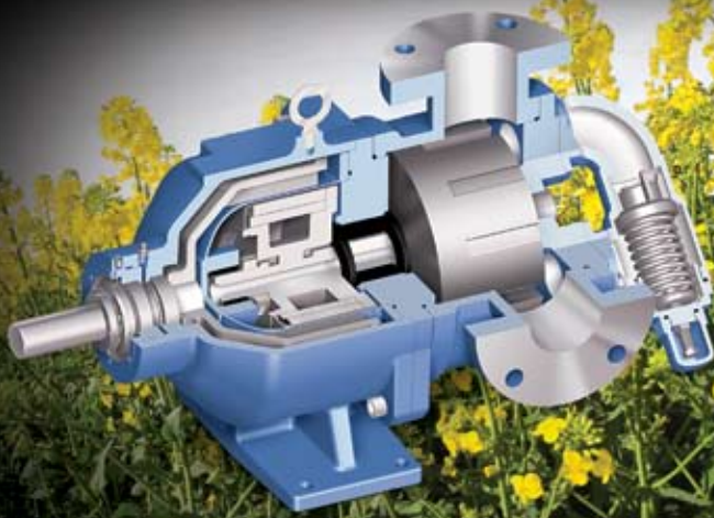
Universal Mag Drive Internal Gear Pump
