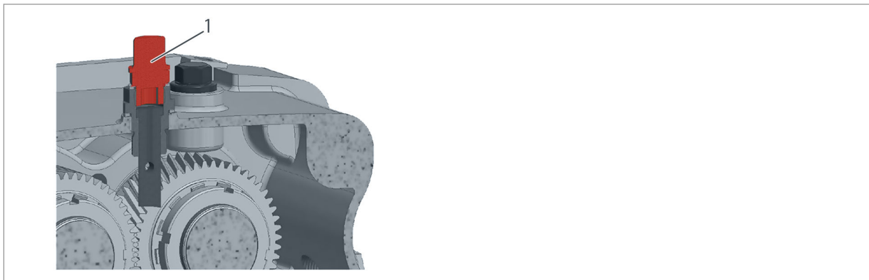
Fig. 10: Ventilation filter on the bearing casing
