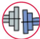
**Mis-aligned pumps** add excess radial loads and stresses to shafts, bearings and seals. This is one of the most common causes of premature pump failure. Liquiflo's **Close-Coupled** option was designed to eliminate the need of having to manually align the pump and motor. Using our **Close-Coupled** option, you simply bolt the pump and motor together and exact **alignment is guaranteed**.
