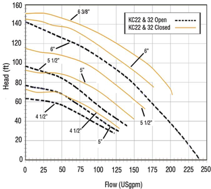
50 Hz, 2900 rpm - KC22 & 32, Open & Closed Impellers
