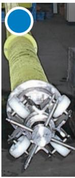
CATAG, a Hydra-Cell distributor, was asked to design and produce a complete washing system to clean pipes after welding and before a coating process... for a fabrication plant in Egypt. The recycled water used is abrasive as it contains weld spatter particles up to 500 microns in size and had previously caused problems with centrifugal pumps. A Hydra-Cell pump with ceramic valves and seats handles the fluid well without undue wear.
