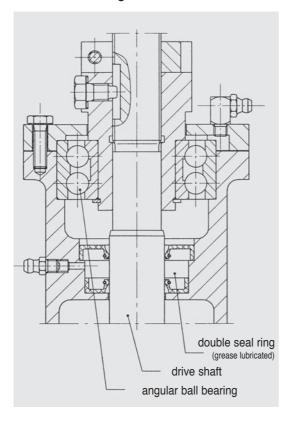
The drive shaft is fixed axially through a grease-lubricated, double-row angular ball bearing. This ball bearing carries the rotor weight and the residual thrust loads. A grease lubricated double seal ring protects the bearing from shaft sealing leakage.
