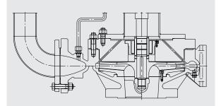
Design with open impeller
