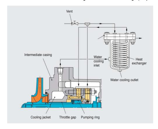
Circulation leads from a pumping ring over the seal, through a water cooled heat exchanger and back to the seal chamber. The cooling water goes through a cooling jacket in the intermediate casing and through the heat exchanger.
