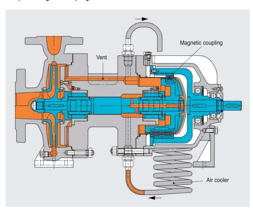
Besides common sealed pumps also sealless pumps with magnetic coupling can be used for hot water. The termination of the main wear part (the mechanical seal) lead to considerably longer "mean time between failure" and therefore higher availability. Hot water spill through seal failure is also excluded. The pump design is self-venting and does not require water cooling.
