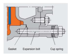
Centerline mounted design according to API 610 / ISO 5199 is available for high operating temperatures on request.
