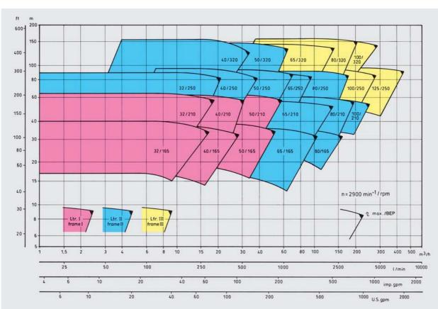
Performance curves of the individual pump sizes, also for 1750 / 3500 rpm, with NPSH-values and power consumption, are available on request.
