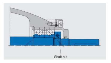
The roller bearings takes the remaining hydraulic radial loads. The bearings proved a life time of more than 25000 operating hours even under severe conditions.
