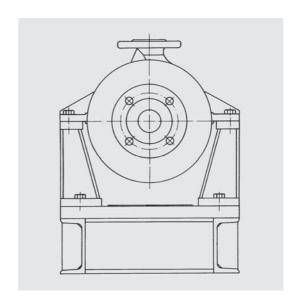
All of the HPL / HPR-pumps will generally be provided with centerline mounted casings.
