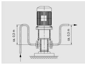
During the suction phase – when priming the empty suction line – the side-channel pumps build up a gas/liquid mixture. The gas or air will be separated and pressed into the pressure pipe while the operating liquid returns to the pump. It is therefore necessary to install the piping in a way that the operating liquid can remain in the pump.
