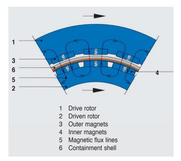
The drive rotor with the drive magnets is keyed to the motor shaft, the driven rotor with the driven magnets is keyed to the pump shaft.
