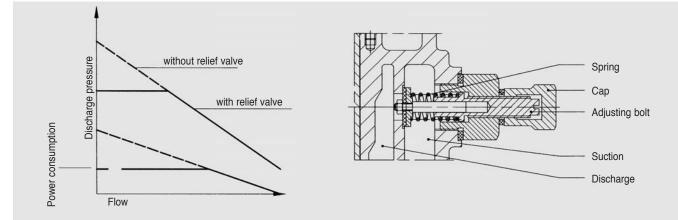
Contrary to centrifugal pumps, the side channel pumps generate a steep head rise and an increased power consumption at lower flow rates.
