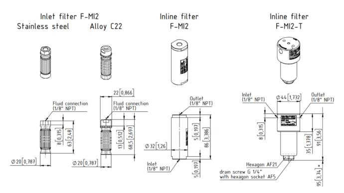
\* Servicing height for filter element exchange
