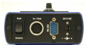
A switch enables local or remote control via the top-mounted potentiometer or the rear 0–10 V external signal or RS-232 for a PC.
