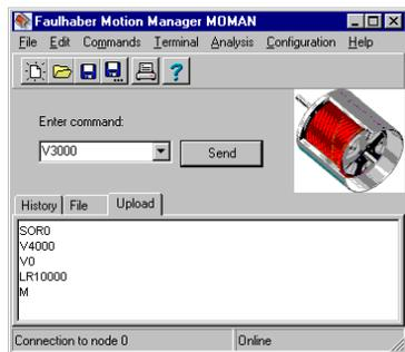
All motor parameters for pump control can be set and saved with the Windows® software »Motion Manager«. The program language is ASCII-based. Dosage programs can easily be typed on a computer and transferred to the EEPROM.
