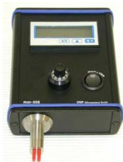
The top panel includes an on/off switch and a fine tuning potentiometer for manual flow control. A low pressure series pump is mounted inside the chassis.
