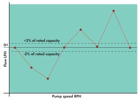
Q1 = Measured Flow at set point speed 600 rpm API 675 REF ±3% of Rated Capacity
