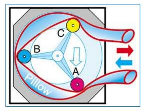
The pillow volume determines the roller-step volume which depends on:
