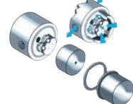
This type of pump head design has a seal plate mounted with a deliberate play in the suction part of the pump chamber (hence the expression Suction Shoe). Discharge pressure keeps the Suction Shoe seated tightly on top of the gears which prevents flow from decreasing in high-pressure applications.
