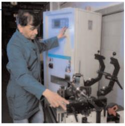
Technician balancing inner magnet for a mag-drive pump: Precision balancing of internal components significantly extends the service life of our products.
