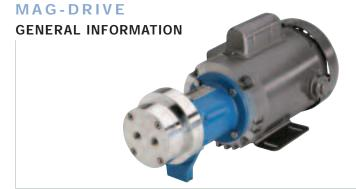
Liquiflo's **4-Series** pumps are low-flow magnetically-driven external gear pumps that are completely field repairable. The 4-Series housings are manufactured from Bar Stock in 316 Stainless Steel, Alloy-C or Titanium. With several material options for shafts, gears, wear plates and bearings, these pumps can be used in a wide variety of chemical processing applications.
