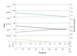
FLOW RATE NOMINAL: 40 mL/min (@ 2.8 Bar, 3V) FLOW RATE MAX: 94 mL/min (@ 0 Bar, 5V)
