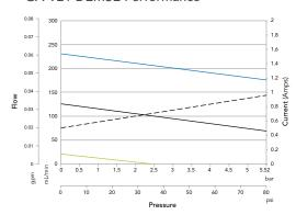
FLOW RATE NOMINAL: 90 mL/min (@ 2.8 Bar, 3V) FLOW RATE MAX: 231 mL/min (@ 0 Bar, 5V) **DISPLACEMENT:** 0.042 mL/rev
