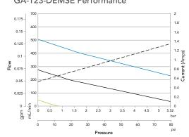
FLOW RATE NOMINAL: 110 mL/min (@ 2.8 Bar, 3V) FLOW RATE MAX: 506 mL/min (@ 0 Bar, 5V)
