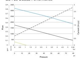
FLOW RATE NOMINAL: 1000 mL/min (@ 2.8 Bar, 3V) FLOW RATE MAX: 3190 mL/min (@ 0 Bar, 5V)
