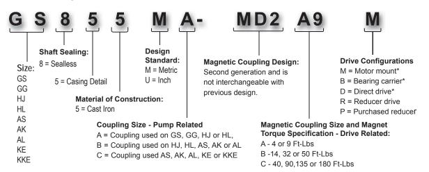
\*To assure the proper bracket and outer magnet is supplied on an M unit (Motor Mounted Drive), the motor frame (NEMA or IEC) must be specified when ordering. For B and D drives, specify the shaft style (inch or metric) that will be required for proper mounting on the unit.
