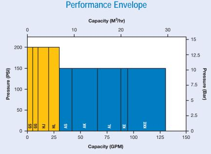
Note: Capacities to 38 M3/hr (167 gpm) and/or pressures to 14 bar (200 psi) may be allowable with engineering review.
