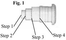
Note: ALWAYS use a 1" I.D. hose properly secured to the barb spout using a hose clamp.
