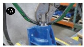
Plastic Air Valve - Remove and replace o-rings. Insert cap (item 6) push down until groove for the retaining ring is visible. Make sure to lubricate the o-rings prior to inserting into the valve body with a compatible lubricant.
