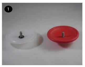
2 For Santoprene fitted pumps place the inner plate (item 23) over the bolt so that the round groove in the inner plate faces the diaphragm. For PTFE fitted pumps place the small diaphragm o-ring (item 22) into the groove of the diaphragm. Then place the inner plate over the bolt so that the round groove in the inner plate faces the diaphragm.
