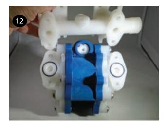
3 Stand the pump upright onto the suction manifold feet (item 12). Press the valve balls (item 15), valve seats (item 14), and seat o-rings (item 13) into the discharge manifold (item 16) in the same order as the suction side was done in step 11. Place the discharge manifold atop the pump, tighten, and torque the discharge manifold bolts (item 11) in an "X" pattern. Torque to 50 in-lbs (5.6 N-m).
