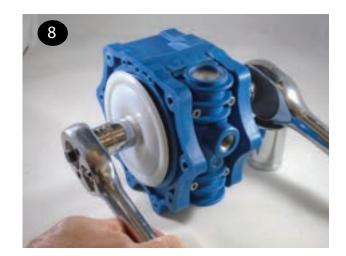
9 Install the liquid chambers (item 18) by placing one side over the diaphragm. Start all 6 screws (item 11) before tightening and torqueing. Torque all fasteners in a star pattern to 50 in-lbs (5.6 N-m). Start all 5 screws (item 17) before tightening and Torqueing. Torque all screws in a X Pattern to 30 in-lbs (3.4 N-m). Repeat to install the second liquid chamber. Ensure both chambers are orientated the same and that the inlet and outlet ports are vertical when facing the front of the pump.
