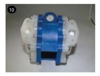
Press the valve seats (item 14) into the seat bore then the valve seat o-rings (item 13) into the groove that is formed by the seats.
