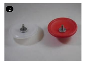
3 Apply a medium strength thread locker, such as Loctite® 246, to the outer plate (19) bolt threads and shaft (item 27) threads. To ensure thread locker cures quickly, a primer such as Loctite® SF7649 should be used. Thread the shaft onto the outer plate bolt until it is snug.
