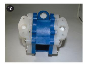
11 Place the valve seats (item 14) into the seat bore then the valve seat o-rings (item 13) into the groove that is formed by the seats.
