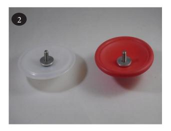
3 Apply a medium strength thread locker, such as Loctite® 246, to the outer plate (19) bolt threads and shaft (item 27) threads. To ensure thread locker cures quickly, a primer such as Loctite® SF7649 should be used. Thread the shaft onto the outer plate bolt until it is snug.
