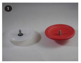
Process Santoprene fitted pumps place the inner plate (item 23) over the bolt so that the round groove in the inner plate faces the diaphragm. For PTFE fitted pumps place the small diaphragm o-ring (item 22) into the groove of the diaphragm. Then place the inner plate over the bolt so that the round groove in the inner plate faces the diaphragm.
