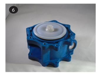
The other diaphragm(s) (item 17) and inner/outer plates (items 19 & 23) can be installed onto the opposite end of the shaft (item 27). It may be easier to thread the molded in bolt into the shaft if the diaphragm(s) is inverted on one or both sides. This can be done by hand.
