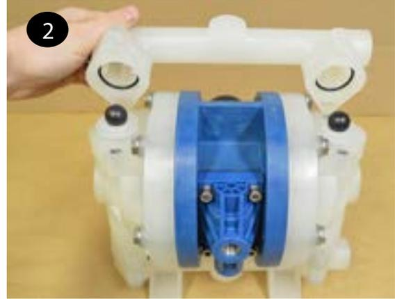
**3** Repeat the above steps for the suction manifold (item 12). The seat o-rings, valve seats and valve balls (items 13, 14, 15 & 16) are located in the liquid chambers (item 18).
