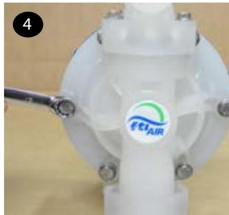
**5** To remove the diaphragms (items 20/ 21), begin by loosening the (2) outer plates (item 19) using 2-20mm wrenches. Use 6-sided sockets or wrenches to prevent damage to the hex portion of the outer plate.
