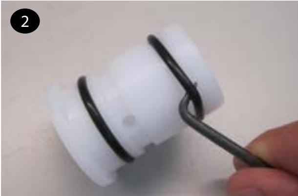
**2** Aluminum Air Valve - Remove and replace o-ring (item 5). Install cap (item 6), tighten, and torque the valve cap screws (item 7). Repeat for the remaining cap.
