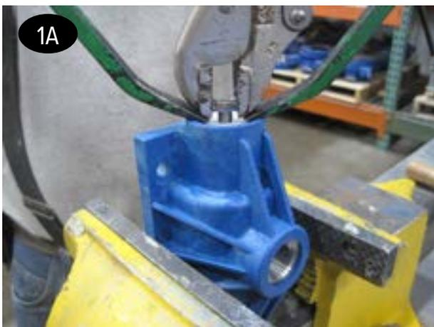
**1** Aluminum Air Valve - To replace the valve cap o-rings (item 5), remove the (3) button head cap screws (item 7) using a 3mm hex wrench.
