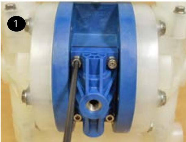
**2** Pull the valve body and gasket (items 3 & 30) off the front of the center section (item 28) and the muffler plate gasket, muffler plate and muffler (items 29, 31 & 33) off the back.
