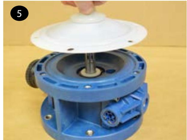
**6** The other diaphragm(s) (items 20/21) and inner/outer plates (items 19 & 22) can be installed onto the opposite end of the shaft (item 27). It may be easier to thread the molded in bolt into the shaft if the diaphragm(s) is inverted on one or both sides. This can be done by hand.
