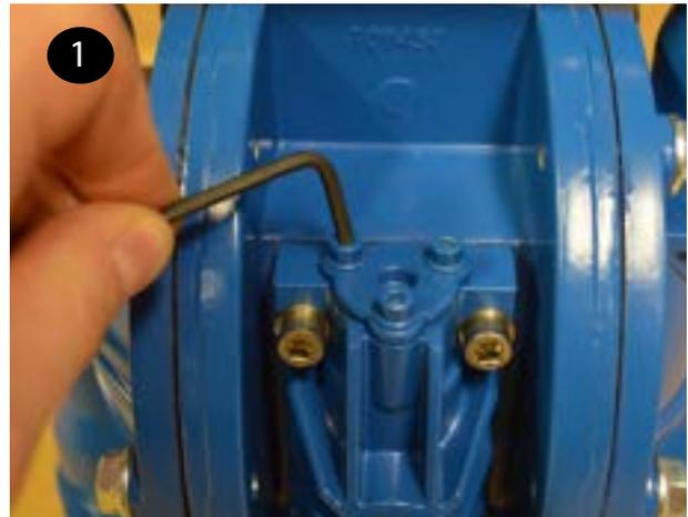
**2** Plastic Air Valve - Remove and replace o-ring (item 5). Insert cap (item 6) and push down until groove for the retaining ring is visible. Make sure to lubricate the o-rings prior to inserting into the valve body with a compatible lubricant.
