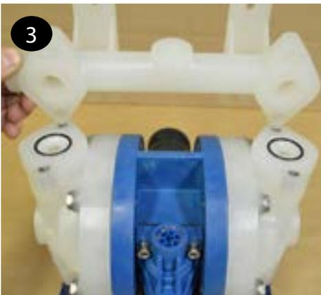
**4** Remove both liquid chambers by removing the (6) bolts (items 17) on each liquid chamber using a 13mm (or 1/2") wrench. Inspect and replace diaphragms if needed.
