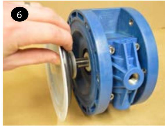
7 To remove the remaining diaphragm(s) (items 20/21) and plates (items 19 & 22) from the shaft (item 27), place the shaft in a vise fitted with soft jaws. Using a 6-sided 20mm wrench, remove the remaining diaphragm(s) and plates. Soft jaws are required to prevent damaging the shaft. A damaged shaft will result in accelerated o-ring wear. Jaws can be fitted with wood, plastic, rubber, or other soft material to prevent shaft damage.
