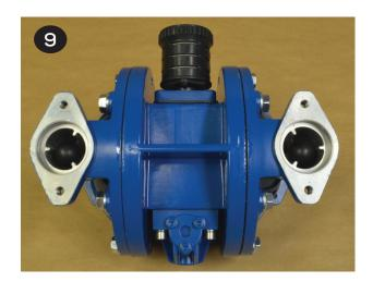
install (1) of the valve seat o-rings (item 13) into the liquid chamber (item 17) followed by the valve seat (item 14) and then another valve seat o-ring (item 13). The o-ring will fit into the groove created by the valve seat and liquid chamber.
