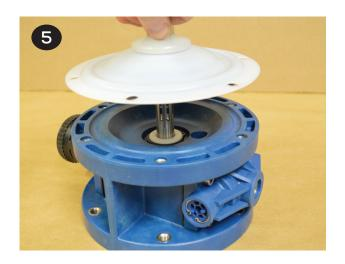
The other diaphragm(s) (items 20/21) and inner/outer plates (items 18 & 22) can be installed onto the opposite end of the shaft (item 27). It may be easier to thread the molded in bolt into the shaft if the diaphragm(s) is inverted on one or both sides. This can be done by hand.
