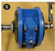
Remove the outer plate, diaphragm(s), and inner plate (items 18, 20/21 & 22) from the side that is loosened. Pull or push the shaft (item 27) and remaining plates and diaphragms out of the center section. If pulling, it may be easier to grip the diaphragm if it is inverted.
