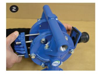
Place the new gasket (item 30) on the air valve (item 3) and ensure the slots in the gasket align with the slots in the air valve and valve plate (item 10).
