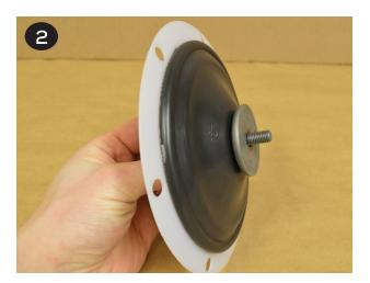
Apply a couple drops of a medium strength thread locker, such as Loctite® 246, to the outer plate bolt (item 19). Thread the shaft (item 27) onto the bolt until it is snug to the flat back side of the inner plate (item 22).
