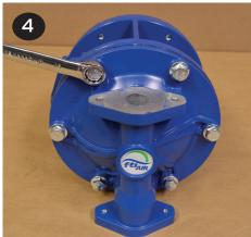
To remove the diaphragms (items 20/21), begin by loosening the (2) outer plates (item 18) using 2-20mm wrenches. Use 6-sided sockets or wrenches to prevent damage to the hex portion of the outer plate.
