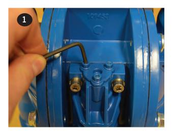
Plastic Air Valve - Remove and replace o-ring (item 5). Install cap (item 6) and tighten until groove for the retaining ring is visible.
