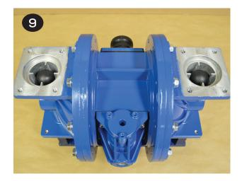
Install the valve seat o-rings (item 13) into both sides of the valve seat (item 14). Install the valve seats into the liquid chambers. Valve seats are symmetrical.
