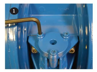
Plastic Air Valve - Remove and replace o-rings (item 5). Insert cap (item 6) and push down until groove for the retaining ring is visible. Install retaining ring. Make sure to lubricate the o-rings prior to inserting into the valve body with a compatible lubricant. **Aluminum Air Valve** - Remove and replace o-ring (item 5). Install cap (item 6), tighten, and torque the valve cap screws (item 7). Repeat for the remaining cap.
