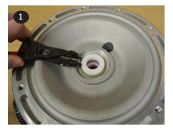
Use the supplied grease packets to lightly grease the OD and ID o-rings (items 23 & 26) that come preinstalled in the new shaft bushing supplied in air end kits. Insert the shaft bushing into the center section (item 28) and reinstall the retaining ring.
