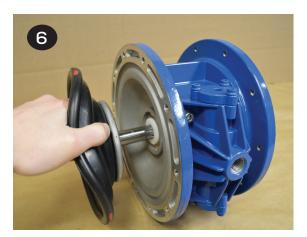
To remove the remaining diaphragm(s) (items 20/21) and plates (items 18 & 22) from the shaft (item 27), place the shaft in a vise fitted with soft jaws. Using a 6-sided 30mm wrench, remove the remaining diaphragm(s) and plates. Soft jaws are required to prevent damaging the shaft. A damaged shaft will result in accelerated o-ring wear. Jaws can be fitted with wood, plastic, rubber, or other soft material to prevent shaft damage.
