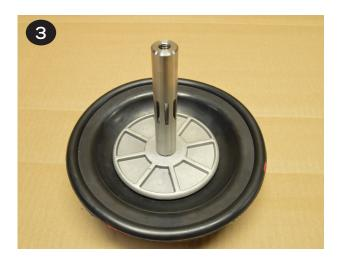
The shaft (item 27) and shaft o-rings (item 26) should retain the lubricant that was factory applied. If they appear dry, apply a light coat of lithium thickened grease. Avoid over lubrication as it can cause decreased performance of the air distribution system.
