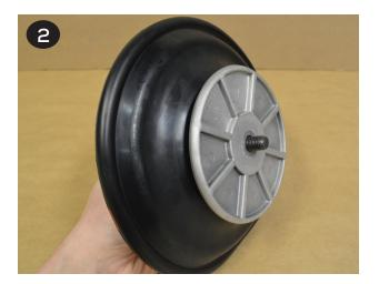
Apply a couple drops of a medium strength thread locker, such as Loctite<sup>®</sup> 246, to the cast/threaded outer plate bolt (item 19). Thread the shaft (item 27) onto the bolt until it is snug to the flat back side of the inner plate (item 22).
