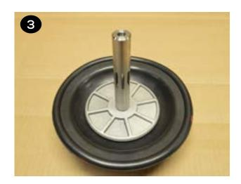
4 The shaft (item 27) and shaft o-rings (item 26) should retain the lubricant that was factory applied. If they appear dry, apply a light coat of lithium thickened grease. Avoid over lubrication as it can cause decreased performance of the air distribution system.
