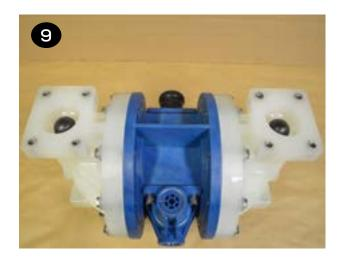
Place the valve seats (item 15) into the seat bores of the liquid chambers (item 18). The ring gland in the valve seat (item 15) should be facing away from the valve ball. Install the valve seat o-rings (item 13) into the valve seats.
