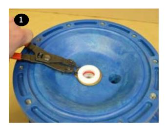
Use the supplied grease packets to lightly grease the OD and ID o-rings (items 23 & 26) that come preinstalled in the new shaft bushing supplied in air end kits.
