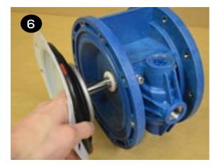
To remove the remaining diaphragm(s) (items 20/21) and plates (items 19 & 22) from the shaft (item 27), place the shaft in a vise fitted with soft jaws. Using a 6-sided 30mm wrench, remove the remaining diaphragm(s) and plates. Soft jaws are required to prevent damaging the shaft. A damaged shaft will result in accelerated o-ring wear. Jaws can be fitted with wood, plastic, rubber, or other soft material to prevent shaft damage.
