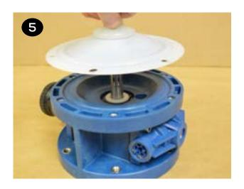
The other diaphragm(s) (items 20/21) and inner/outer plates (items 19 & 22) can be installed onto the opposite end of the shaft (item 27). It may be easier to thread the molded in bolt into the shaft if the diaphragm(s) is inverted on one or both sides. This can be done by hand.
