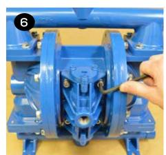
**6** Tighten and torque the (4) cap
