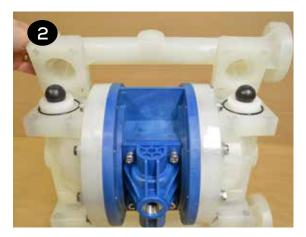
Repeat the above steps for the suction manifold (item12). The seat o-rings, valve seats and valve balls (items 13, 14, 15 & 16) are located in the liquid chambers (item 18). Remove both liquid chambers by removing the (10) bolts (items 17) on each liquid chamber using a 13mm (or ½") wrench. Inspect and replace diaphragms if needed.
