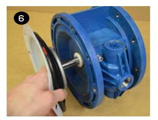
To remove the remaining diaphragm(s) (items 20/21) and plates (items 19 & 22) from the shaft (item 27), place the shaft in a vise fitted with soft jaws. Using a 6-sided 30mm wrench, remove the remaining diaphragm(s) and plates. Soft jaws are required to prevent damaging the shaft. A damaged shaft will result in accelerated o-ring wear. Jaws can be fitted with wood, plastic, rubber, or other soft material to prevent shaft damage.
