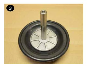
• The shaft (item 27) and shaft o-rings (item 26) should retain the lubricant that was factory applied. If they appear dry, apply a light coat of lithium thickened grease. Avoid over lubrication as it can cause decreased performance of the air distribution system.
