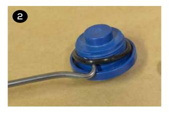
**Aluminum Air Valve** - Remove and replace o-ring (item 5). Install cap (item 6), tighten, and torque the valve cap screws (item 7). Repeat for the remaining cap.
