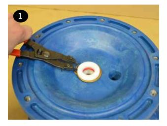
Use the supplied grease packets to lightly grease the OD and ID o-rings (items 23 & 26) that come preinstalled in the new shaft bushing supplied in air end kits.
