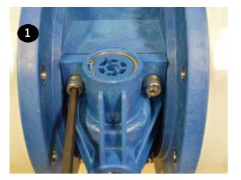
Pull the valve body and gasket (items 3 & 30) off the front of the center section (item 28) and the muffler plate gasket, muffler plate and muffler (items 29, 31 & 33) off the back.
