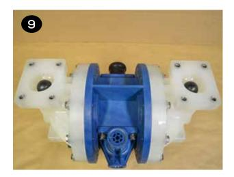
Place the valve seats (item 15) into the seat bores of the liquid chambers (item 18). The ring gland in the valve seat (item 15) should be facing away from the valve ball. Install the valve seat o-rings (item 13) into the valve seats. Place the manifold o-rings (item 14) into the o-ring gland on the suction manifold (item 12). Place the suction manifold atop the pump and install, tighten, and torque the (8) manifold bolts (item 11).
