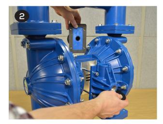
• Place the new gasket (item 38) on the air valve (item 3) and ensure the slots in the gasket align with the slots in the air valve and valve plate (item 10).
