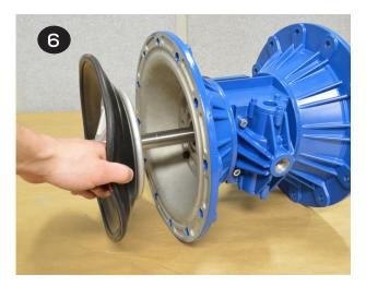
To remove the remaining diaphragm(s) (items 21/22) and plates (items 19 & 23) from the shaft (item 32), place the shaft in a vise. Using a 6-sided 30 mm wrench, remove the remaining diaphragm(s) and plates.
