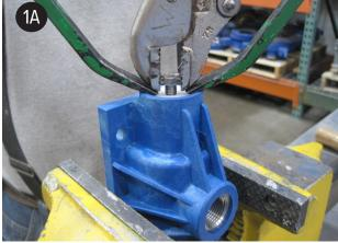
• Aluminum Air Valve - To replace the valve cap o-rings (item 5), remove the (3) button head cap screws (item 7) using a 5 mm hex wrench.
