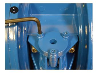
Plastic Air Valve - Remove and replace o-ring (item 5). Insert cap (item 6) and push down until groove for the retaining ring is visible. Install retaining ring. Make sure to lubricate the o-rings prior to inserting into the valve body with a compatible lubricant.
