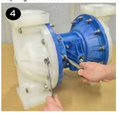
To remove the diaphragms (items 21/22), begin by loosening the (2) outer plates (item 20) using two 30 mm wrenches. Use 6-sided sockets or wrenches to prevent damage to the hex portion of the outer plate.
