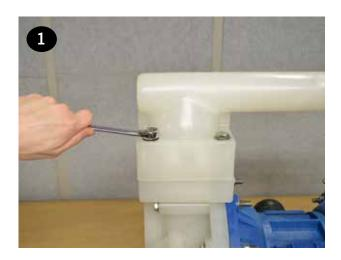
The discharge seat o-rings, valve seats, and valve balls (items 14, 15, 16, & 17) can now be accessed and replaced if needed.
