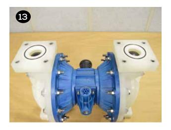
Place the manifold o-rings (item 15) into the o-ring gland on the suction manifold (item 39). Place the suction manifold atop the pump and install, tighten and torque the (8) manifold bolts & washers (items 11 & 12).
