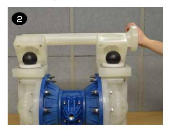
Repeat the above steps for the suction manifold (item13). The seat o-rings, valve seats and valve balls (items 14, 15, 16, & 17) are located in the liquid chambers (item 19).
