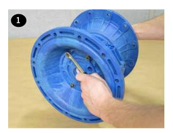
Remove and set aside the air valve (item 3) using a 6 mm hex wrench (see "Valve & Muffler Gasket Replacement" section for more details). The shaft bushings (item 29) can be removed by placing a large socket between the two bushings. Place an extension into the socket from one side of the center section. Tap with a rubber mallet to remove the bushing. Repeat for the remaining bushing.
