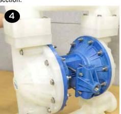
Place the muffler gasket (item 37) over the (4) cap screws & lock washers (items 1 & 2) on the back side of the center section (item 35) followed by the muffler plate and muffler (items 38 & 41).
