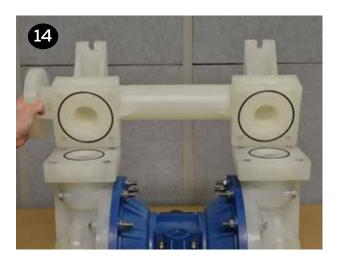
Stand the pump upright onto the suction manifold feet (item 13). Place the large o-rings (item 15) into the glands in the face of the liquid chambers (item 19) followed by the small o-ring (item 14) in the gland of the valve seats (item 16). Place the valve seats on the liquid chambers with the o-ring down against the liquid chamber.
