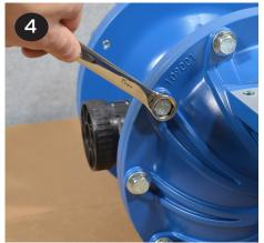
• To remove the diaphragms (items 20/21), begin by loosening the (2) outer plates (item 19) using 2-30mm wrenches. Use 6-sided sockets or wrenches to prevent damage to the hex portion of the outer plate.
