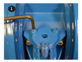
Plastic Air Valve - Remove and replace o-ring (item 8). Insert cap (item 9) and push down until groove for the retaining ring is visible. Install retaining ring. Make sure to lubricate the o-rings prior to inserting into the valve body with a compatible lubricant. **Aluminum Air Valve** - Remove and replace o-ring (item 8). Install cap (item 9), tighten, and torque the valve cap screws (item 10). Repeat for the remaining cap.
