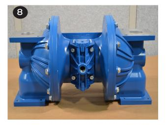
Flip the pump upside down and drop the suction valve balls (item 16) into the liquid chamber (item 18) ball cages.
