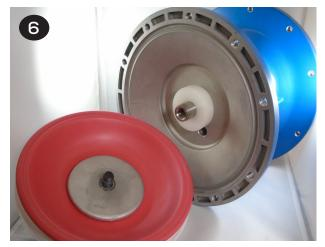
Tighten and torque the outer plates (item 19) to 81.4 N-m (720 in-lbs).
