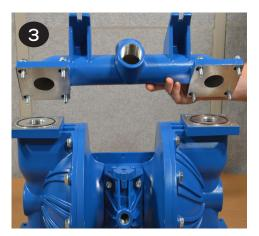
• Remove both liquid chambers (item 18) by removing the (10) bolts (item 17) on each liquid chamber using a 15 mm wrench. Inspect and replace diaphragms if needed.
