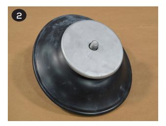
3 Apply a couple drops of a medium strength thread locker, such as Loctite® 246, to the cast/ threaded outer plate bolt (item 19). Thread the shaft (item 29) onto the bolt until it is snug to the flat back side of the inner plate (item 22).
