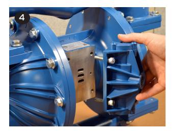
• Tighten and torque the (4) cap screws into the muffler plate to 7.9 N-m (70 in-lbs).
