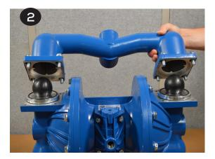
Repeat the above steps for the suction manifold (item13). The seat o-rings, valve seats and valve balls (items 14, 15, & 16) are located in the liquid chambers (item 18).
