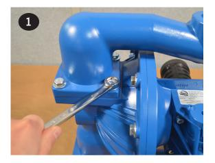
The discharge seat o-rings, valve seats and valve balls (items 14, 15, & 16) can now be accessed and replaced if needed.
