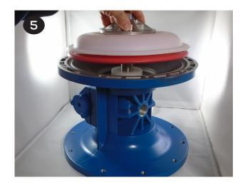
• The other diaphragm(s) (items 20/21) inner/outer plates (items 19 & 22) and bump stop (item 44) can be installed onto the opposite end of the shaft (item 29). It may be easier to thread the bolt into the shaft if the diaphragm(s) is inverted on one or both sides. This can be done by hand.
