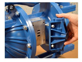
• Place the new gasket (item 6) on the air valve (item 3) and ensure the slots in the gasket align with the slots in the air valve and valve plate (item 5).
