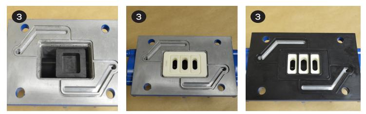
Insert the (4) cap screws & washers (items 1 & 2) through the valve body and gasket (items 3 & 6) and bolt to the center section (item 31). Ensure the slide valve and valve plate (items 4 & 5) are in place and the valve sits flat on the center section.
