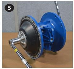
• Remove the outer plate, diaphragm(s), inner plate, bump stop (items 19, 20/21, 22 & 44) from the side that is loosened. Pull or push the shaft (item 29) and remaining plates and diaphragms out of the center section. If pulling, it may be easier to grip the diaphragm if it is inverted.
