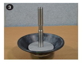
• The shaft (item 29) and shaft o-rings (item 25) should retain the lubricant that was factory applied. If they appear dry, apply a light coat of lithium thickened grease. Avoid over lubrication as it can cause decreased performance of the air distribution system.
