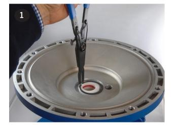
**C** Use the supplied grease packets to lightly grease the OD and ID o-rings (items 23 & 25) that come preinstalled in the new shaft bushing supplied in air end kits.
