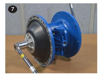
Install the liquid chambers (item 18) by placing one side over the diaphragm. Start all bolts (item 17) before tightening and torqueing. Torque all fasteners in a star pattern to 35.2 N-m (312 in-lbs). Repeat to install the second liquid chamber. Ensure both chambers are oriented in the same direction and that the inlet and outlet ports are vertical when facing the front of the pump as shown.
