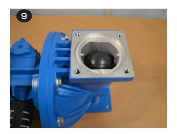
Install the valve seat o-rings (item 14) into both sides of the valve seat (item 15). Install the valve seats into the liquid chambers. Valve seats are symmetrical.
