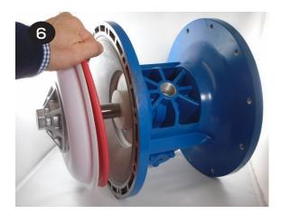
To remove the remaining diaphragm(s) (items 20/21) and plates (items 19 & 22) from the shaft (item 29), place the shaft in a vise fitted with soft jaws. Using a 6-sided 30mm wrench, remove the remaining diaphragm(s) and plates. Soft jaws are required to prevent damaging the shaft. A damaged shaft will result in accelerated o-ring wear. Jaws can be fitted with wood, plastic, rubber, or other soft material to prevent shaft damage.
