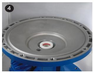
• Push the shaft (item 29) through the bump stop (item 44) and center of the shaft bushing (item 24). It is normal for this to be a tight fit, especially if the shaft and shaft o-rings (item 25) are in good condition.
