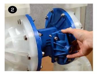
3 Place the new gasket (item 6) on the air valve (item 3) and ensure the slots in the gasket align with the slots in the air valve and valve plate (item 5).
