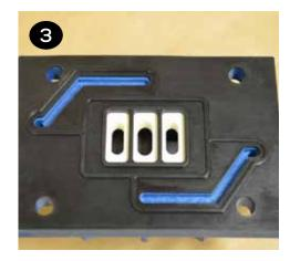
Insert the (4) cap screws (item 1) through the valve body and gasket (items 3 & 6) and place onto the center section (item 35). Ensure the slide valve and valve plate (items 4 & 5) are in place and the valve sits flat on the center section.
