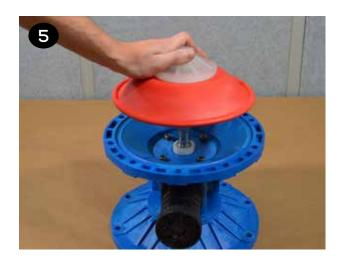
6 It may be easier to thread the molded in bolt into the shaft if the diaphragm(s) is inverted on one or both sides. This can be done by hand.
