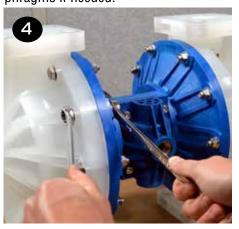
To remove the diaphragms (items 22/23), begin by loosening the (2) outer plates (item 21) using two 30 mm wrenches. Use 6-sided sockets or wrenches to prevent damage to the hex portion of the outer plate.
