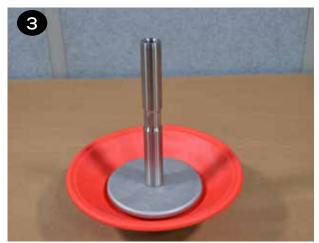
4 The shaft (item 32) and shaft o-rings (item 31) should retain the lubricant that was factory applied. If they appear dry, apply a light coat of lithium thickened grease. Avoid over lubrication as it can cause decreased performance of the air distribution system.
