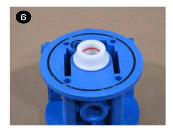
Install both air chambers (item 27) by placing one side on top of the center section (item 35). Ensure the air path hole of the center section lines up with the through hole in the air chamber. Insert the (4) bolts & washers (items 25 & 26) through the air chamber and center section.
