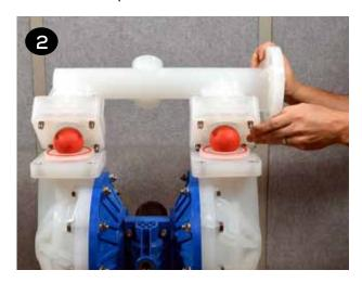
Repeat the above steps for the suction manifold (item14). The seat o-rings, valve seats and valve balls (items 15, 16, & 17) are located in the liquid chambers (item 20).
