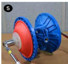
Remove the outer plate, diaphragm(s), and inner plate (items 21, 22/23 & 24) from the side that is loosened. Pull or push the shaft (item 32) and remaining plates and diaphragms out of the center section. If pulling, it may be easier to grip the diaphragm if it is inverted.
