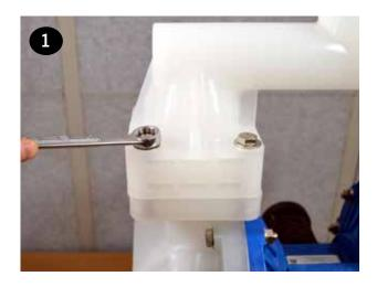
The discharge seat o-rings, valve seats, and valve balls (items 15, 16, & 17) can now be accessed and replaced if needed.
