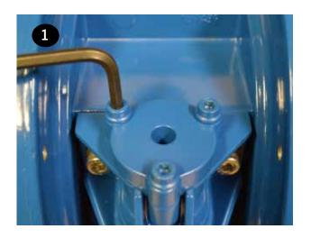
Plastic Air Valve - Remove and replace o-ring (item 8). Install cap (item 9) and tighten until groove for the retaining ring is visible. Install retaining ring (item 10).
