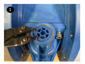
• Aluminum Air Valve - To replace the valve cap o-rings (item 8), remove the (3) button head cap screws (item 11) using a 4 mm hex wrench. Repeat for the remaining cap.
