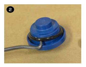
Aluminum Air Valve - Remove and replace o-ring (item 8). Install cap (item 9), tighten, and torque the valve cap screws (item 11). Repeat for the remaining cap.
