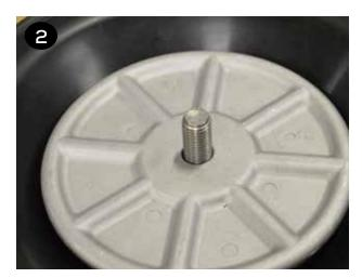
Apply a couple drops of a medium strength thread locker, such as Loctite® 246, to the molded in outer plate bolt (item 21). Thread the shaft (item 32) onto the molded in bolt until it is snug to the flat back side of the inner plate (item 24).
