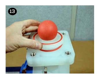
Place the valve balls (item 17) on the valve seats and discharge manifold (item 37) atop the components that are stacked on top of the liquid chambers. Install, tighten and torque the (8) manifold bolts & washers (items 12 & 13).
