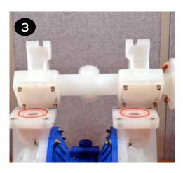
Remove both liquid chambers by removing the (10) bolts, washers & nuts (items 18, 19 & 28) on each liquid chamber using a 17mm wrench and nuts can be removed using a 15mm wrench. Inspect and replace diaphragms if needed.
