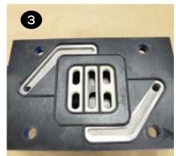
Insert the (4) cap screws & washers (items 1 & 2) through the valve body and gasket (items 3 & 35) and place onto the center section (item 34). Ensure the slide valve and valve plate (items 9 & 10) are in place and the valve sits flat on the center section.
