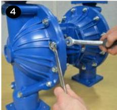
To remove the diaphragms (items 21/22), begin by loosening the (2) outer plates (item 19) using two 30 mm wrenches. Use 6-sided sockets or wrenches to prevent damage to the hex portion of the outer plate.
