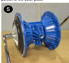
Remove the outer plate, diaphragm(s), and inner plate (items 19, 21/22 & 23) from the side that is loosened. Pull or push the shaft (item 31) and remaining plates and diaphragms out of the center section. If pulling, it may be easier to grip the diaphragm if it is inverted.
