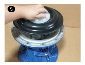
6 It may be easier to thread the bolt into the shaft if the diaphragm(s) is inverted on one or both sides. This can be done by hand.
