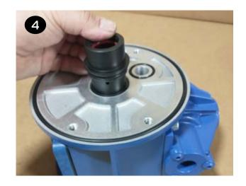
Inspect the shaft (item 31) for damage. It is common for shafts to become grooved during service. Grooving is normally caused by carbonized oil and/or abrasive foreign material getting trapped between the seal and the shaft. Over time, deep grooves can form in the shaft. When that occurs, it is recommended that the shaft be replaced.
