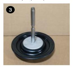
4 The shaft (item 31) and shaft o-rings (item 30) should retain the lubricant that was factory applied. If they appear dry, apply a light coat of lithium thickened grease. Avoid over-lubrication as it can cause decreased performance of the air distribution system.
