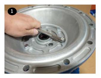
Remove and set aside the air valve (item 3) using a 6mm hex wrench (see Valve and Muffler Gasket Replacement section for more details). The shaft bushings can be removed by placing a large socket between the two bushings. Place an extension into the socket from one side of the center section. Tap with a rubber mallet to remove the bushing. Repeat for the remaining bushing.
