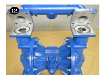
Stand the pump upright onto the suction manifold feet. Place the valve seat o-rings (item 13) into both sides of the valve seat. Place the seat on the liquid chamber (item 18). Place the valve balls (item 15) on the seats and discharge manifold (item 38) atop the components that are stacked on top of the liquid chambers. Install, tighten and torque the (8) manifold bolts (item 11).
