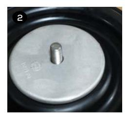
3 Apply a couple drops of a medium strength thread locker, such as Loctite® 246, to the cast/threaded outer plate bolt (item 20). Thread the shaft (item 31) onto the bolt until it is snug to the flat back side of the inner plate (item 23).
