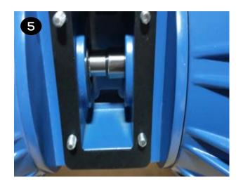
**6** Tighten and torque the (4) cap screws & washers (items 1 & 2) into the muffler plate.
