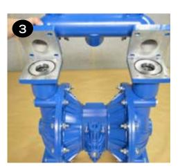
Remove both liquid chambers (item 18) by removing the (12) bolts & nuts (item 16, 17, & 27) on each liquid chamber using a 15 mm wrench. Inspect and replace diaphragms if needed.
