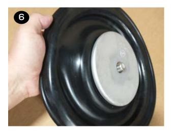
The other diaphragm(s) (items 21/22) and inner/outer plates (items 19 & 23) can be installed onto the opposite end of the shaft (item 31).
