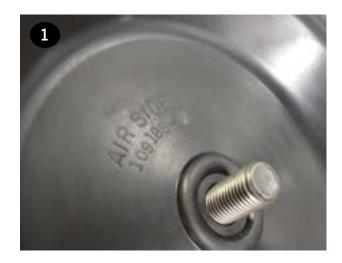
Place the inner plate (item 23) over the cast/threaded bolt. Ensure the round recess in the plate faces the diaphragm (item 22).
