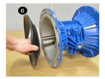
To remove the remaining diaphragm(s) (items 21/22) and plates (items 19 & 23) from the shaft (item 31), place the shaft in a vise. Using a 6-sided 30 mm wrench, remove the remaining diaphragm(s) and plates.
