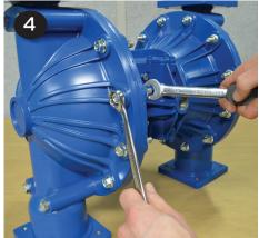
To remove the diaphragms (items 21/22), begin by loosening the (2) outer plates (item 19) using two 30 mm wrenches. Use 6-sided sockets or wrenches to prevent damage to the hex portion of the outer plate.
