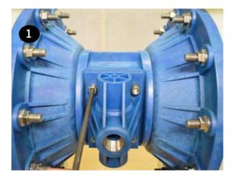
Pull the valve body and gasket (items 3 & 36) off the front of the center section (item 35) and the muffler plate gasket, muffler plate and muffler (items 37, 38 & 41) off the back.
