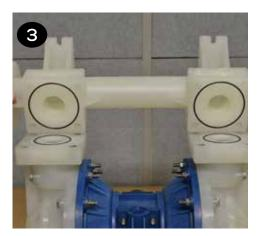
• Remove both liquid chambers by removing the (12) bolts, washers & nuts (items 11, 12, 18 & 27) on each liquid chamber using a 17mm wrench and nuts can be removed using a 15mm wrench. Inspect and replace diaphragms if needed.
