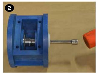
• Use the supplied grease packets to lightly grease the OD and ID o-rings (items 28 & 30) that come preinstalled in the new shaft bushings supplied in air end kits. • Insert both bushings into the center section. Ensure the bushing is fully installed and the large rib on the outside of the bushing is flat against the center section.
