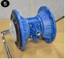
• Remove the outer plate, diaphragm(s), and inner plate (items 20, 21/22 & 23) from the side that is loosened. Pull or push the shaft (item 32) and remaining plates and diaphragms out of the center section. If pulling, it may be easier to grip the diaphragm if it is inverted.
