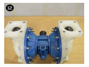
Place the valve seats (item 16) into the seat counter bores of the liquid chambers (item 19). The o-ring (item 14) gland in the valve seat should be facing away from the valve ball.
