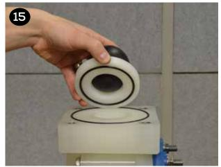
Place the valve balls (item 17) on the valve seats and discharge manifold (item 39) atop the components that are stacked on top of the liquid chambers. Install, tighten and torque the (8) manifold bots & washers (items 11 & 12).
