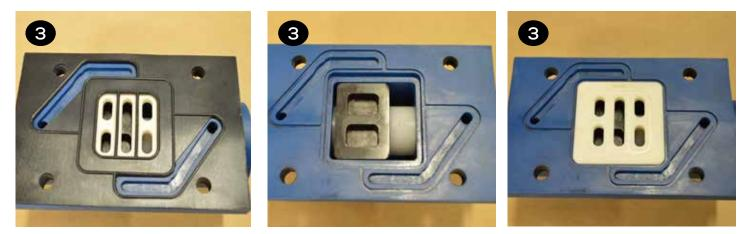
Insert the (4) cap screws (item 1) through the valve body and gasket (items 3 & 36) and place onto the center section (item 35). Ensure the slide valve and valve plate (items 9 & 10) are in place and the valve sits flat on the center section. Place the muffler gasket (item 37) over the (4) cap screws & lock washers (items 1 & 2) on the back side of the center section (item 35) followed by the muffler plate and muffler (items 38 & 41).
