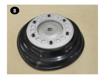
The other diaphragm(s) (items 21/22) and inner/outer plates (items 20 & 23) can be installed onto the opposite end of the shaft (item 30).
