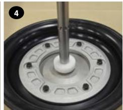
5 The shaft (item 33) and shaft o-rings (item 31) should retain the lubricant that was factory applied. If they appear dry, apply a light coat of lithium thickened grease. Avoid over-lubrication as it can cause decreased performance of the air distribution system.
