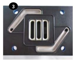
4 Insert the (4) cap screws & washers (items 1 & 2) through the valve body and gasket (items 3 & 37) and place onto the center section (item 36). Ensure the slide valve and valve plate (items 9 & 10) are in place and the valve sits flat on the center section.
