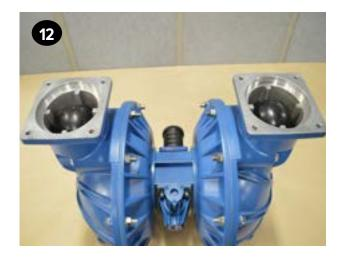
For pumps fitted with metal or PTFE valve seats (item 14), place the valve seat o-rings (item 13) into the glands on both sides of the valve seat. Pumps fitted with rubber or TPE seats do not require valve seat o-rings. All seats are symmetrical, i.e. there is no top or bottom.
