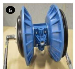
Remove the outer plate, diaphragm(s), and inner plate (items 20, 21/22 & 23) from the side that is loosened. Pull or push the shaft (item 33) and remaining plates and diaphragms out of the center section. If pulling, it may be easier to grip the diaphragm if it is inverted.
