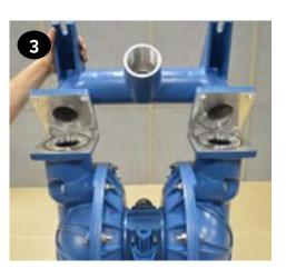
Remove both liquid chambers (item 19) by removing the (10) bolts & nuts (item 16, 18, & 28) on each liquid chamber using a 16 mm wrench. Inspect and replace diaphragms if needed.
