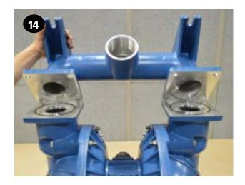
Stand the pump upright onto the suction manifold feet. Place the valve seat o-rings (item 13) into both sides of the valve seat. Place the seat on the liquid chamber (item 19). Place the valve balls (item 15) on the seats and discharge manifold (item 40) atop the components that are stacked on top of the liquid chambers. Install, tighten and torque the (8) manifold bolts (item 11).
