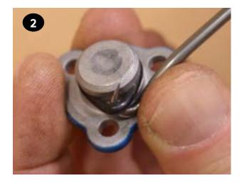
Remove the valve body (item 3) by removing the (4) socket head cap screws and washers (items 1 & 2) that attach the valve body to the muffler plate (item 38) with a 6 mm hex wrench
