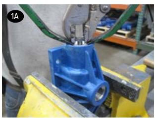
Plastic Air Valve - Remove and replace o-rings (item 5). Insert cap (item 6) and push down until groove for the retaining ring is visible. Install retaining ring. Make sure to lubricate the o-rings prior to inserting into the valve body with a compatible lubricant.
