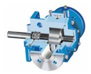
While vane pumps can handle moderate viscosity liquids, they excel at handling low viscosity liquids such as LP gas (propane), ammonia, solvents, alcohol, fuel oils, gasoline, and refrigerants. Vane pumps have no internal metal-to-metal contact and self-compensate for wear, enabling them to maintain peak performance on these non-lubricating liquids. Though efficiency drops quickly, they can be used up to 500 cPs / 2,300 SSU.
